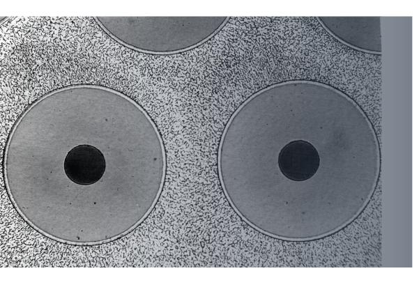
Fiber reinforced Titanium alloy
